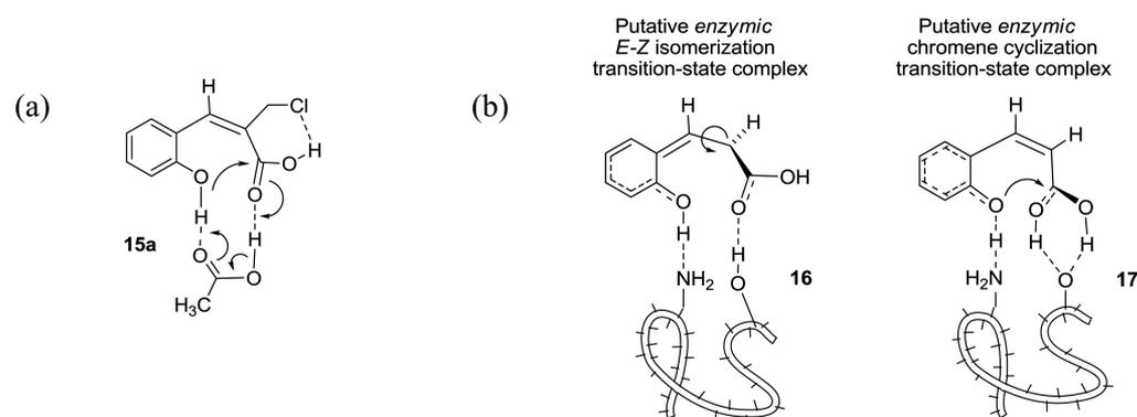
**Figure 12.** (a) Mechanistic depiction of the role of acetic acid as an amphoteric catalyst in the cyclization of (*Z*)-3-(chloromethyl)-2-(hydroxyphenyl)-2-propenoic acid (**15a**). (b) Putative structures involved in a suggested enzyme-catalyzed *E*–*Z* isomerization of *o*-coumaric acid **16** and the subsequent lactonization of the *Z* isomer **17** to form coumarin.
